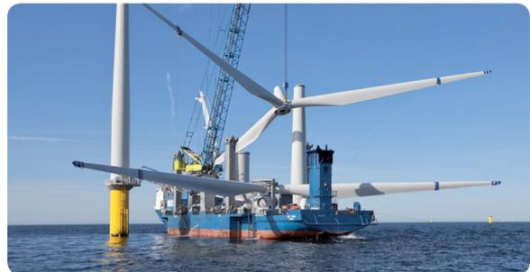
Very heavy foundations, cables and wind turbines will be transported to the wind farm. Some of the components will be delivered at the wind farm, but most of the components will be trucked or shipped to the Port of Grenaa for storage and preparation prior to assembly.
